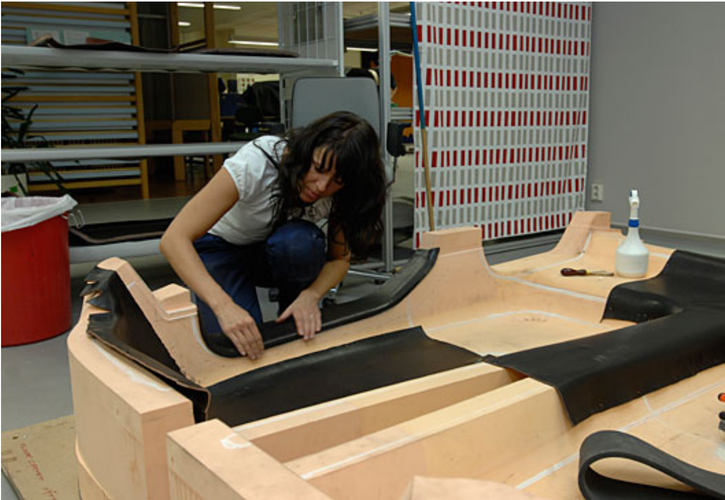
At work on the Volvo production floor lining the XC60 concept car in dark-brown saddle-quality leather. © Volvo Car Corporation
